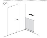
The ideal starting point for installation of the tiles is a corner, ideally square. stick the product to the wall without creating joints: boiserie and mosaic tiles must be laid butt-jointed .
