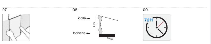
Install the elements, ensuring that adhesive does not come out, thus preventing adhesive getting onto the leather. If adhesive comes out, clean it off immediately using a clean, dry cloth. Alternatively, wait until the adhesive is completely dry (3 days) and remove with your fingers, ensuring mechanical detachment. (as with silicone).
