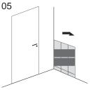
The ideal starting point for installation of the tiles is a corner, ideally square, chosen at the tiling expert's discretion. stick the product to the wall without creating joints: boiserie and mosaic tiles must be laid edge to edge.
